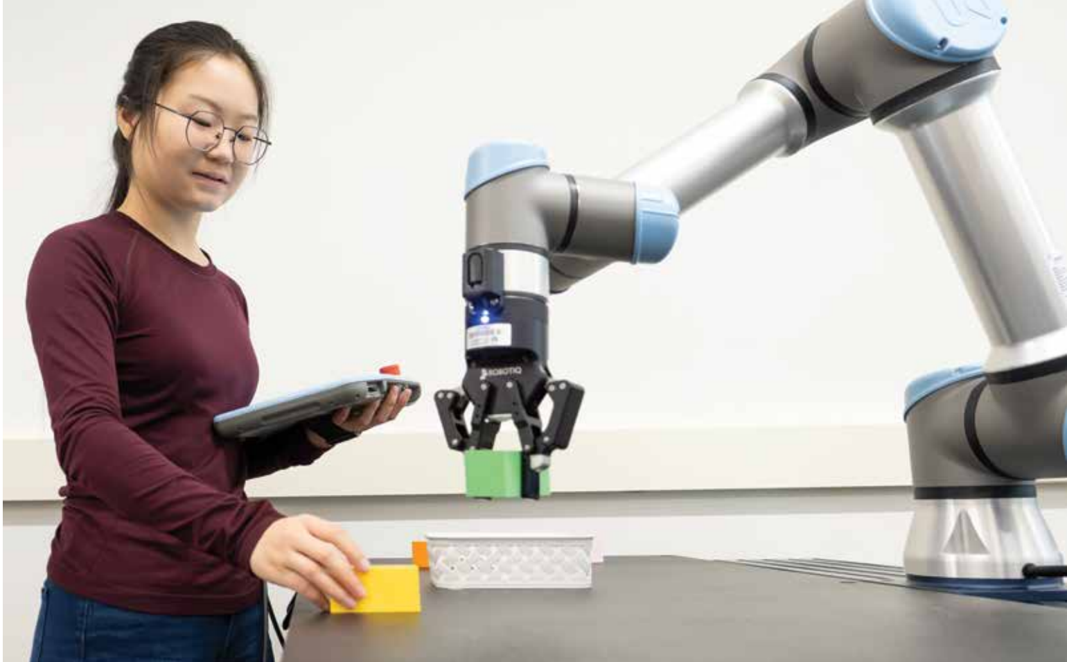
Engineering student, Yuezhen, completing a collaborative robotics experiment, operating and monitoring a robotic arm and performing object manipulation tasks using a tablet controller.
