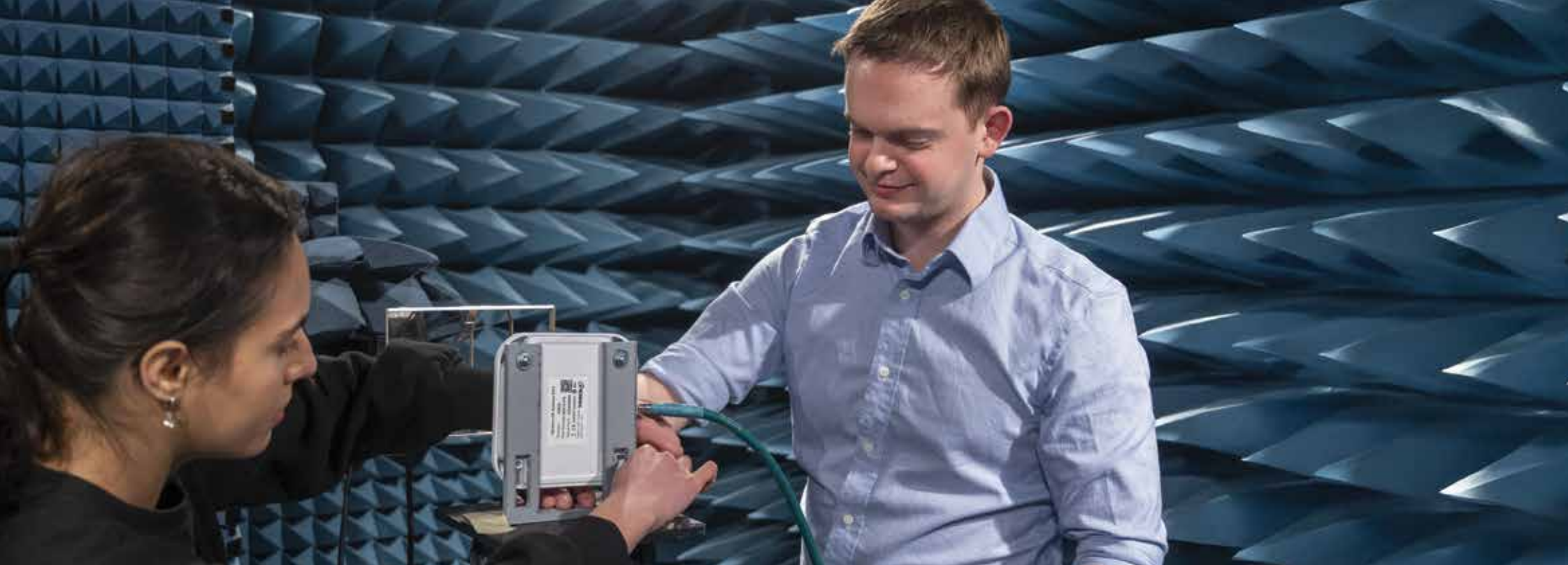
PhD student Christopher and MSc student Romina preparing antenna measurements in the M3 Laboratory's near-field anechoic chamber.
