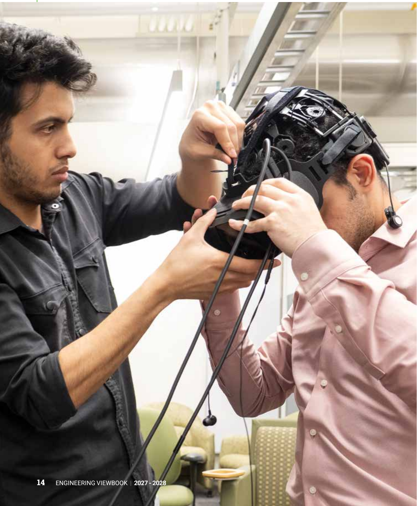
Engineering students, Eren and Mohammad, conducting a neurotechnology experiment, setting up an electroencephalogram (EEG) headset.
